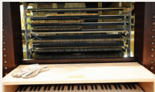
[TOP] Workers install the Opus 135 organ in Auer Concert Hall at the IU Jacobs School of Music. [BOTTOM LEFT] Installation of one of the organ's keyboards. [BOTTOM RIGHT] Detail of the organ's Kowalshyn Servo-pneumatic Lever, which provides a pneumatic assist to the keyboard when using multiple sets of pipes.
